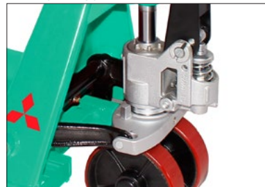
#3 Integrated ACBF* pump has heavy-duty construction for durability and features overload protection. * Only on 540 x 1150.
