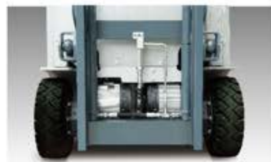
Front wheel dual drive motors offer provide more power.
